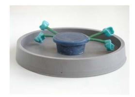
To prevent air bubbles it is important that the parts are fixed with the open side on top or at least parallel to the mould socket base.
