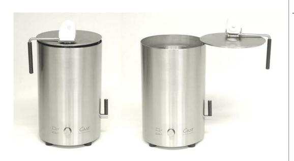
Lift the top lid **2** by turning the lever **13** upward and turn it to the side. The mould holder inside the device must not be able to rotate free by hand operation. In case the mould holder rotates free proceed as indicated in the troubleshooting section.
