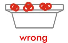
It is important to avoid sprueing to a center sprue base but to mount each sprue radially to the waxdisk. To avoid turbulences and insufficient flow the sprues should be fixed side by side without any overlap (see illustration above).
