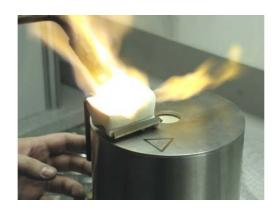
After reaching the liquidus point of the metal it may be pourred into the mould by turning the crucible holder handle 13 in a smooth move to tip over the crucible 11.
